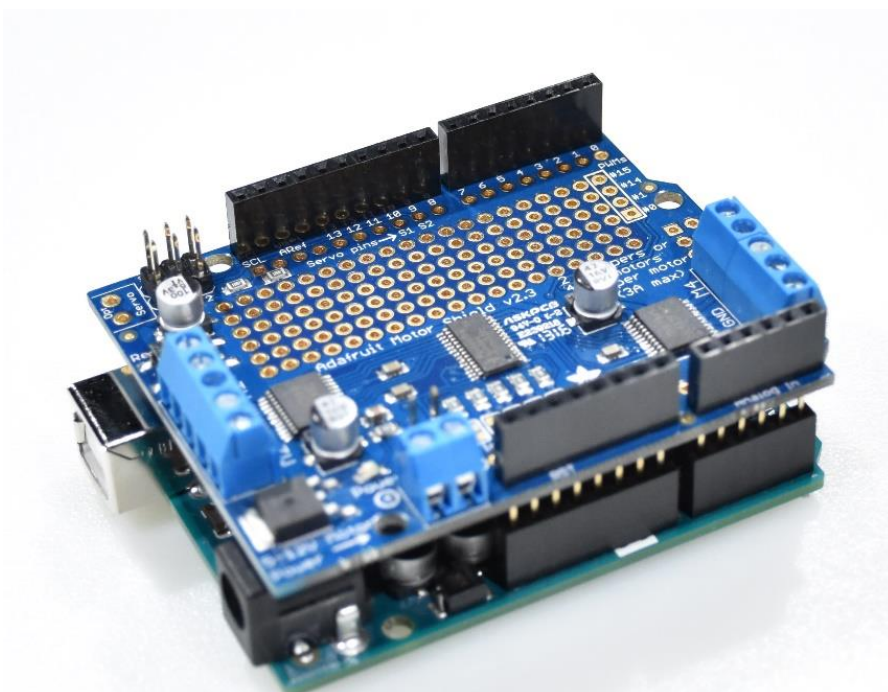
Figure 4-17. Connect the Adafruit Motor/Stepper/Servo Shield on top of the Arduino UNO. Make sure that the connecting pins are properly aligned with the headers of the Arduino UNO.
