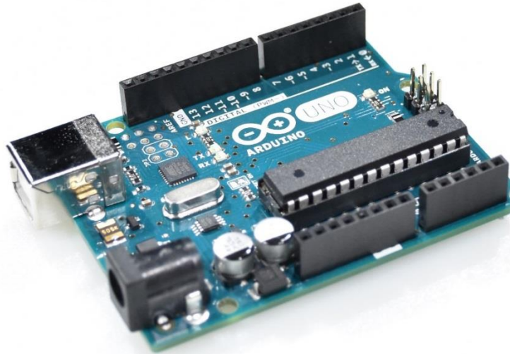
Figure 4-16. The base of the complete stack is the Arduino UNO.
