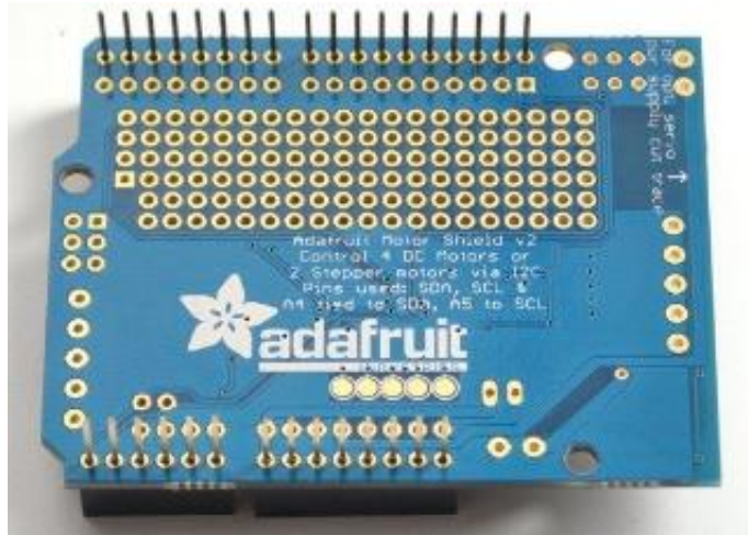
Figure C-2. Start by sliding the 10-pin, the two 8-pin and the 6-pin stacking headers into the outer rows of the top side of the shield. Then flip the board over so that it is resting on the four headers.
