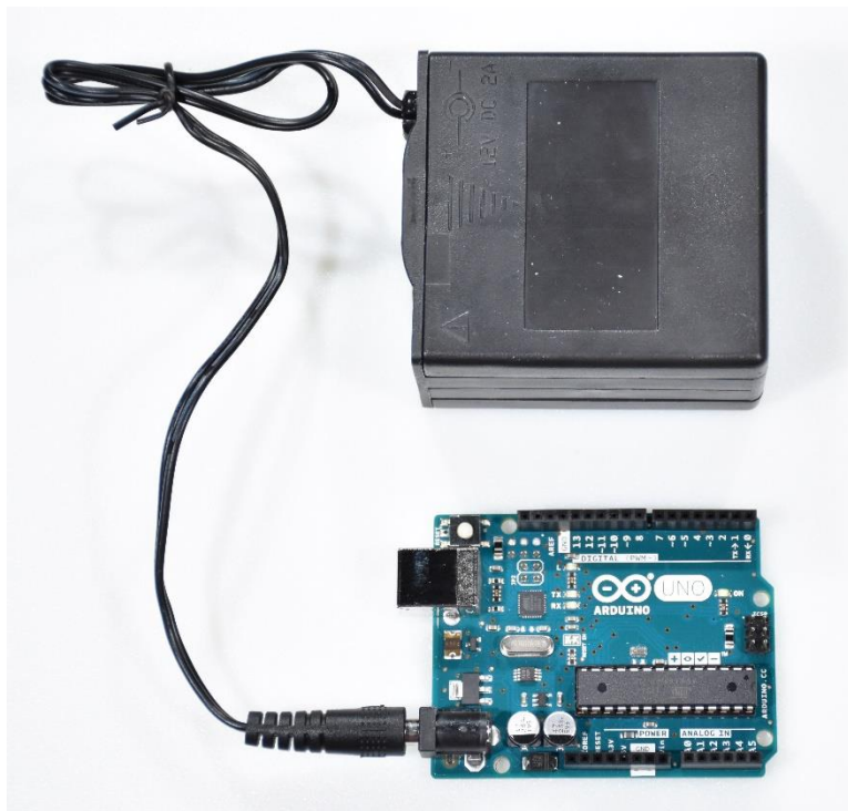
Figure 2-3. Powering the Arduino using a barrel jack, 12V 8AA battery pack.
