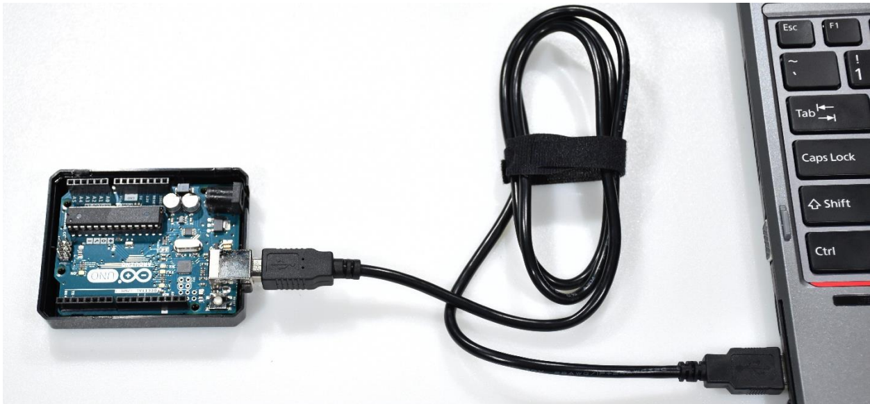
Figure 2-2. Powering the Arduino using a USB cable.
